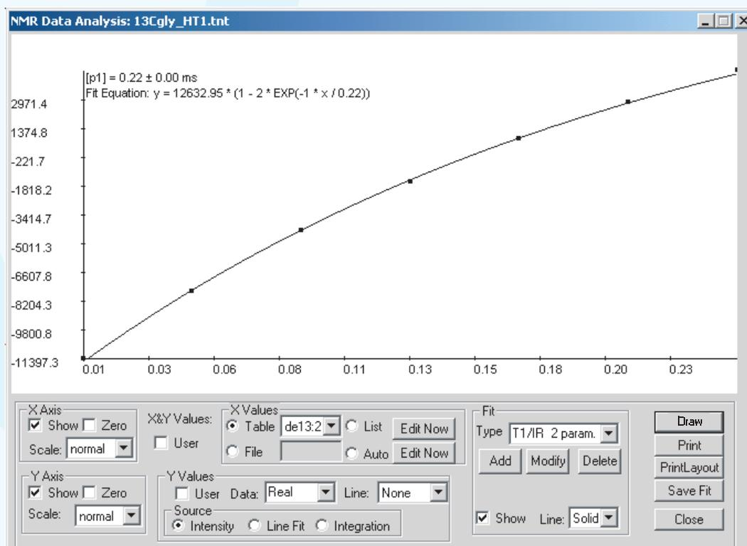
Fig. 3. T<sub>1</sub> fitting for glycine-1-<sup>13</sup>C in the "NTNMR Data Analysis" window. Fitting results: T<sub>1</sub> = 0.22 ms.
